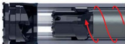
1.) Drive the pilot bit through the casing tube
