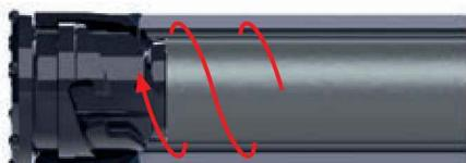
2.) Rotate to locked position in the ring bit
